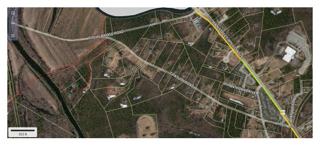
The map below shows the proposed sidewalk (orange) continuing up to the Baptist Church, where there is currently an unmarked crosswalk to the sidewalk on the eastern side of Rte. 119. This crosswalk should be marked and the deteriorated existing sidewalk would need to be replaced, which is why it is shown in orange.
