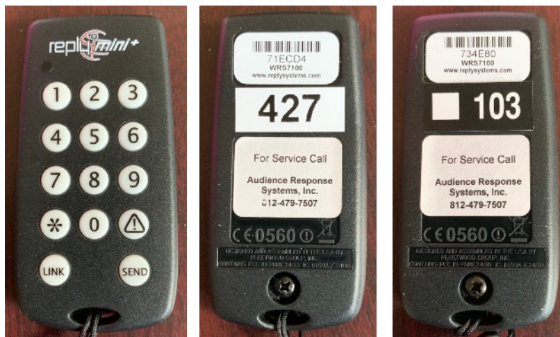
Figure 4: WRS7100 Keypad (L to R) Front, Original (Channel 1) Back, New (Channel 8) Back
