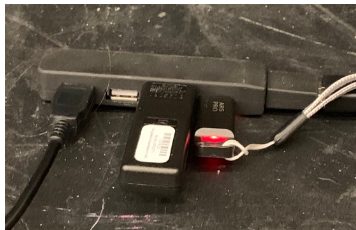
Figure 5: USB Hub With (L to R) Cable to WRS970, WRS971 and HASP
