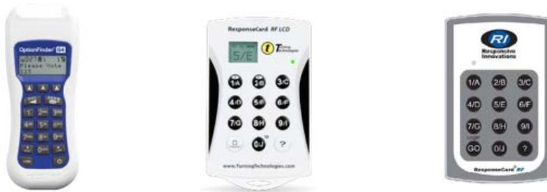
The exact layout of the device depends on the specific system, but they usually include several input buttons, and often a screen or LEDs to provide feedback to the voter. In considering handset options, the committee will require a device containing a screen that provides positive confirmation to the user that the vote was properly sent and recorded.
