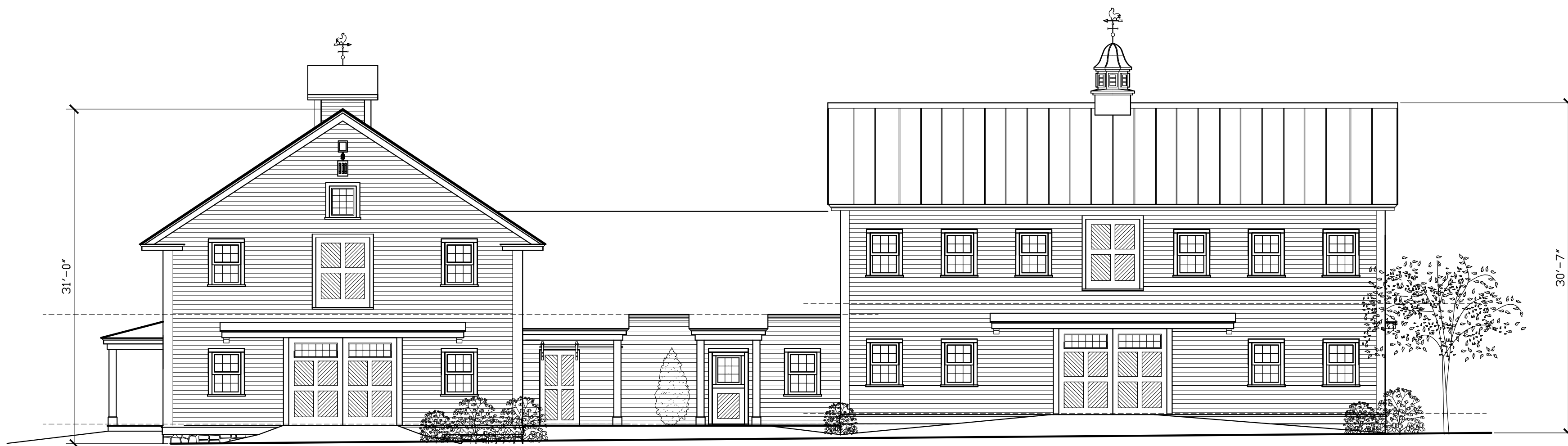
B PROPOSED STABLES REAR ELEVATION A-2 SCALE: 1/8" = 1'-0"
