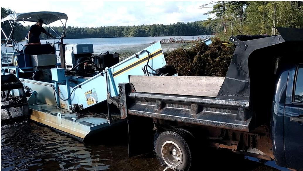
Fig. 2 – Transferring harvested weeds
