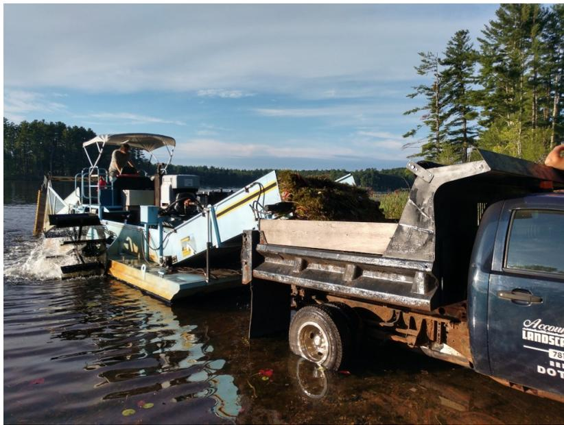
Fig. 1 - The Weed Harvester loading the truck with Fanwort
