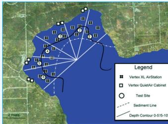
In July 2004, (8) Vertex Air 3 XL systems were installed by Tri-County Aquatics in a 160 acre cove of the 900 acre lake. At the time of installation, muck measurements with a "sludge judge"
