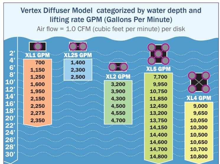
Lifting rates represent total water flow as recorded in both independent testing and real world data collected by Vertex from installed aeration systems. Lifting rate varies significantly by air flow, water depth and other factors.
