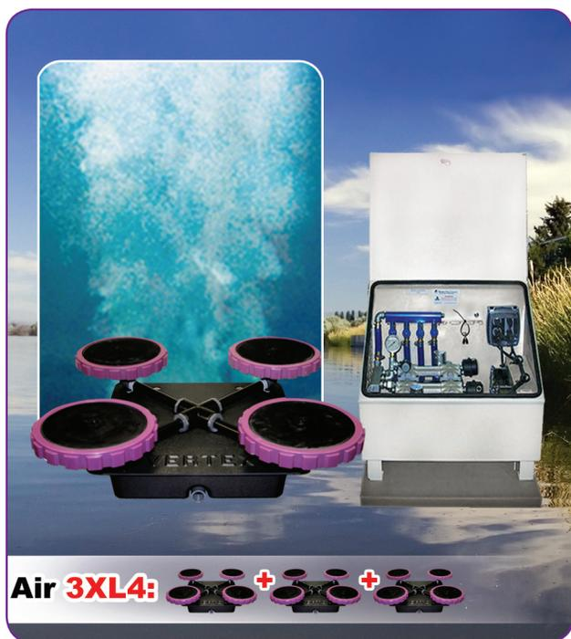
The Vertex Air3 XL4™ pond aerator is a super-efficient, affordable and safe system. In a typical pond, an Air3 XL4™ can aerate approximately 4-7 acres depending on shape, slope, oxygen demand and other factors. Two 1/2hp (0.75kW) Brookwood™ SafeStart™ compressors, housed in our rustproof aluminum outdoor cabinet, feed three bottom mounted XL AirStations™ utilizing Vertex's MicronBubble™ technology.
