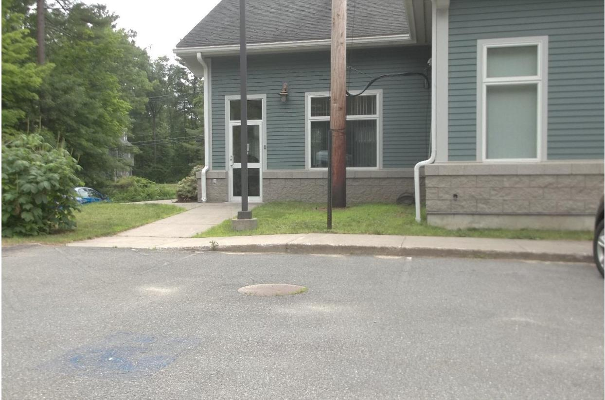
We recommend the town install one van accessible HP parking spot at The Lost Lake Fire Station. The ADA Access Guidelines (ADAAG) require that one space should be a "Van Accessible" space, 8-foot-wide with an 8-foot access aisle and van accessible sign.
